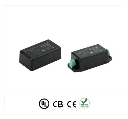
The 56YMR30-xx Series is a performance-focused 30W Encapsulated AC/DC PCB Mount Power Supply. Designed for use in applications such as network equipment and signal distribution hardware. This series is supplied with a Pin or Screw Terminal input connection and supports input voltages of 85~305V AC 47-63Hz.
